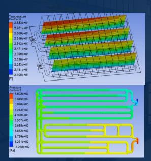
Pack level cooling capacity control, Cell temperature difference in system <2°C
